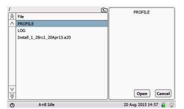
Touch on the file called "Install\_1\_28rc1\_20Apr15.a20", and touch 'Open'. Genie® II will then restart on its own and install the software.
