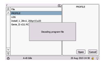
The selected file will be uploaded to Genie® II. When it has finished, a message will be displayed on screen to say "Reset required" at which point turn the machine OFF and ON.
