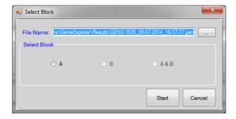
On clicking 'Run' this box will appear. This allows selection of which block is being used and also options for saving of the run file. The default location for saving the files is set within Genie® Explorer, and can be changed in 'Options'.
