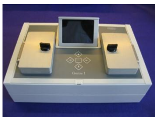
Figure 1: The GENIE detection system allows real-time LAMP and is designed for use with LAMP assays. It has two independent heating blocks that can each process 1-8 samples and can perform temperature gradient.
